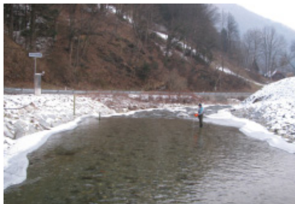
Slika 4. Hidrometrične meritve pretokov na Bistrici in Radoljni sedmega in osmega januarja 2009 (Foto:arhiv ARSO) Figure 4. Current meter measurements on the rivers Bistrica and Radoljna on 7 and 8 January 2009 (Photo: EARS)
